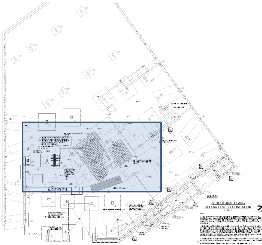
Figure 3 shows the extent of the micro piles on the structural cellar plan
